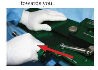
While holding the pin at the bottom, rotate it to the upright and locked position.
