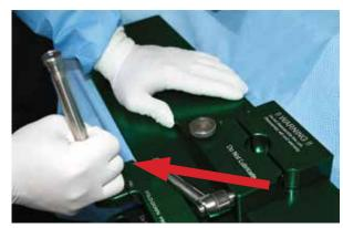
Repeat with the other pin and seat both pins into the Clamp.
