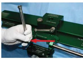
To lower the pin, grab the pin at the bottom and pull the pin creating a gap at the pin base.
