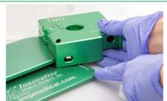
Using your fingers screw in the threaded rod with attached L Plate into the carriage until a boot ball fits into the carriage.
