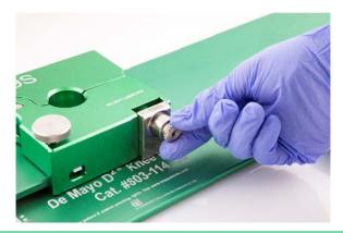
2. Slide the carriage toward the "Loading End" of the Base Plate and slide the carriage around the curved end of the top plate.
