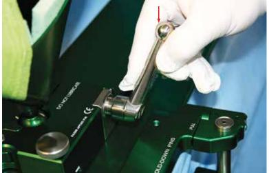
rotate the Handle counterclockwise to the 2:00 o'clock position and release.
