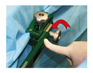
Loosen the side Knob all the way by turning it counter clockwise.
