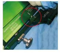
To seat the Base Plate on the Extention, line up the white arrows on the Base Plate and Extension.
