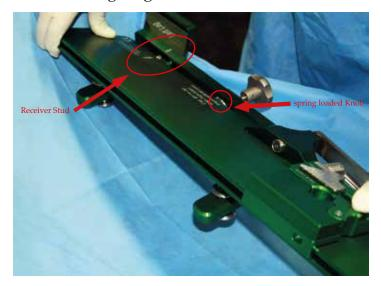
Push down on the Base Plate for final seating, and finger tighten the Knob turning clockwise.
