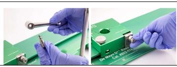
2. Slide the carriage toward the right hand side of the baseplate and slide the carriage around the curved end of the top plate.
