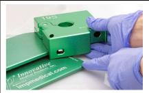
2. Using your fingers screw in the threaded rod with attached L Plate into the carriage until a boot ball fits into the carriage.
