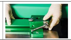
Remove the handle and E-Break for cleaning
